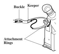
3. Thread the end of the strap back through the keeper and buckle making sure it is threaded under the outer strap. Make sure the strap is not twisted.
